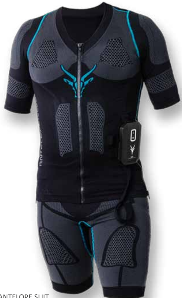
ANTELOPE.SUIT With Moss Embroidered Electrodes for Electrical Muscle Stimulation [2]
