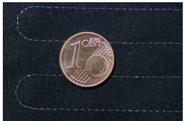
Embroidered Copper wire (70 \mu\text{m} )
